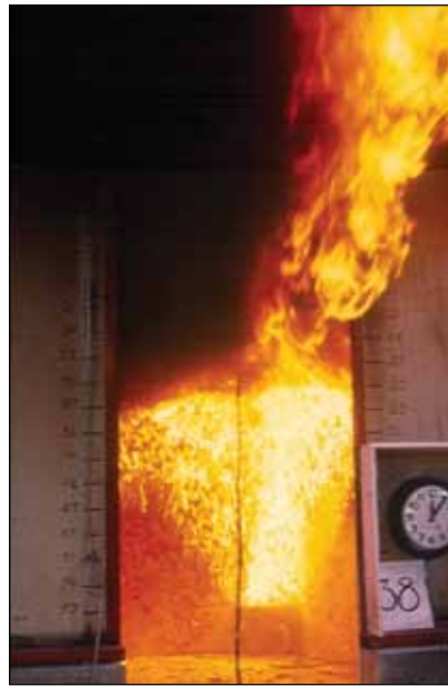
Figure 18-1. Flashover in standard room test.
