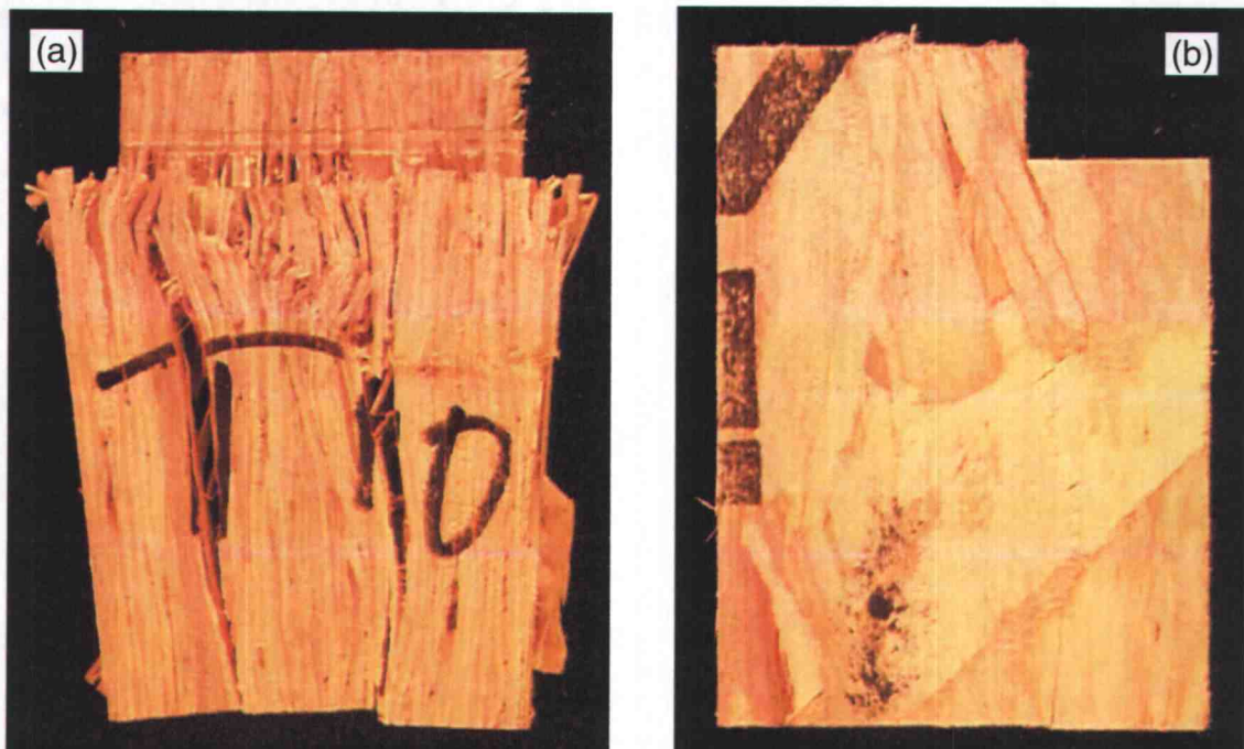
Figure 4-10: Typical Compression Failure in Joist-Oriented LSL Block
